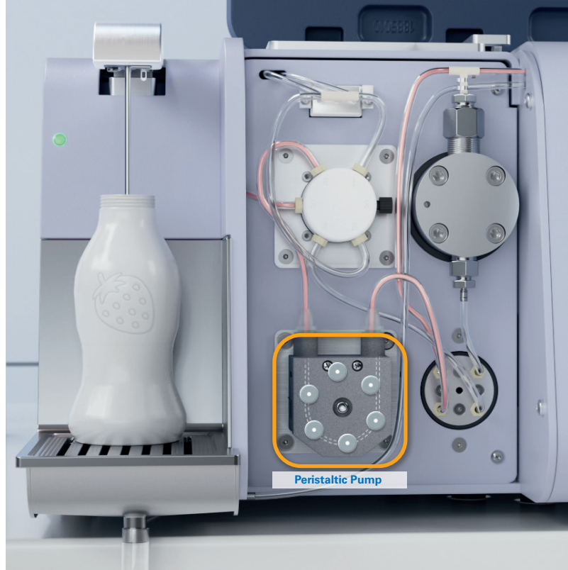
Different sample guidance through the MOVE-T spectrometer with homogenisation of raw milk (left) and peristaltic pumping of other samples (right).
