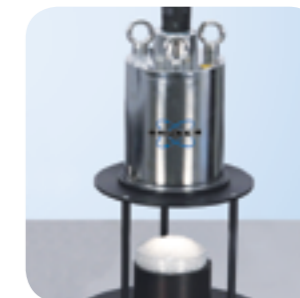
Sensor head is placed on the laboratory mount for offline measurements.
