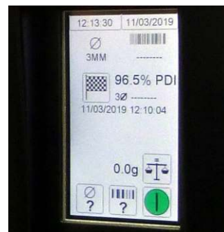
PDI results recorded and displayed on the new colour LCD touch screen
